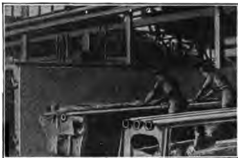
FIG. 189.—Making Cores for Cast Iron Pipe. Cores for pipes are made on a bar. Hay is wound on this bar and then loam is carefully worked into the hay. The core is then dried and given a second coat of mud, dried again, and blackened. It is then placed in the mold.
